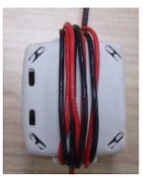
5 Connect the power cables from the power supply to the connector on the rail-UIO-IOTA power conditioning PWA
