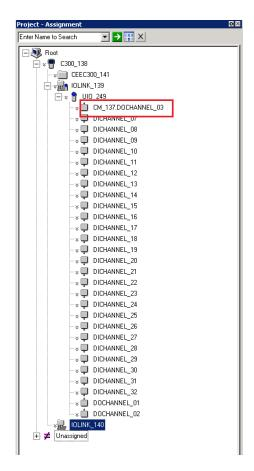
Figure 188: Appearance of DO channels after ganging
