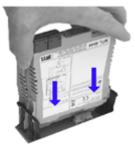
Figure 244: Mounting a module onto an IOTA
