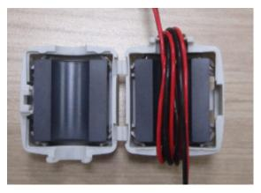
e Lock the ferrite clamp as shown in the following figure.
