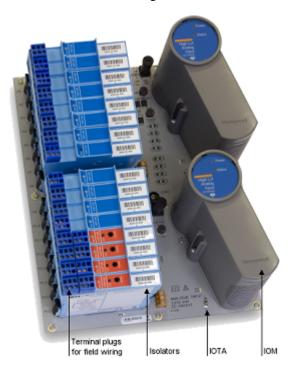
Figure 241: GI/IS board assembly
