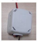
f A Ferrite clamp with 4 turns wound together as shown in the following figure.
