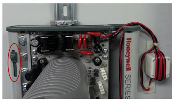
2 Slide the rail-mounted UIO module assembly towards the right to disengage from the DIN rail and remove it.
