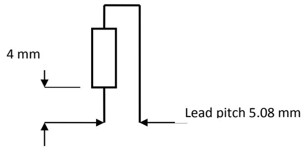
**Figure 12 Resistor Forming**
