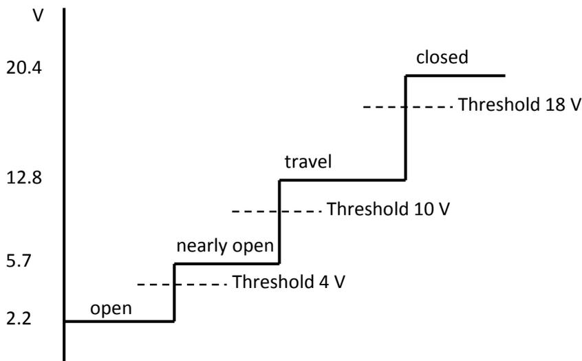
Figure 9 Voltage Input with Limit Switch Position
