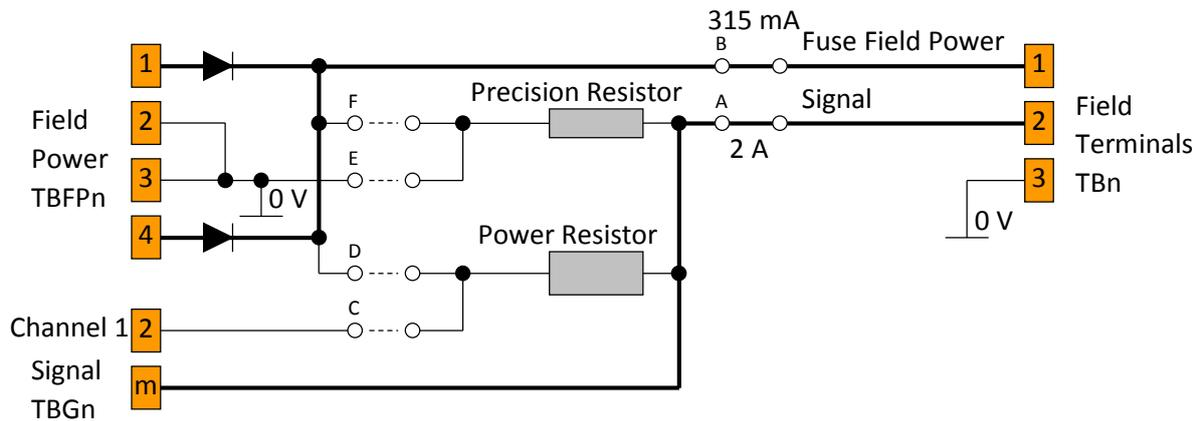
**Figure 4 Digital Inputs (Line Monitored without power)**
