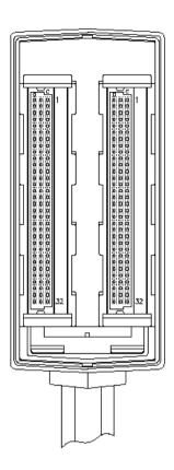
**Figure 3 Expander Processor Cable**
