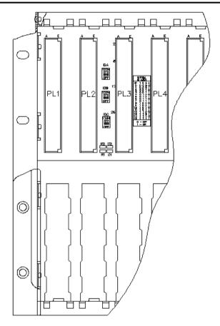
**Figure 2 Expander Processor Slots**
