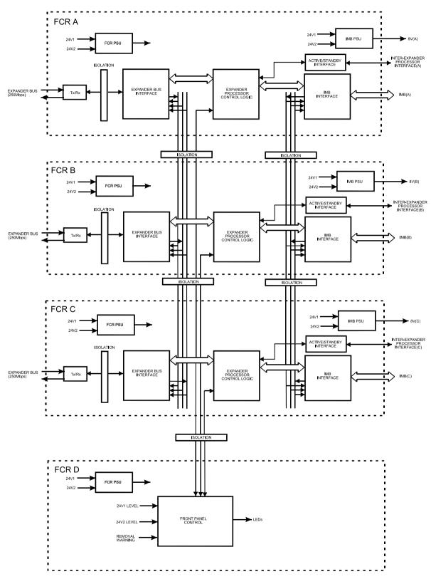
Figure 1 Simplified Block Diagram
