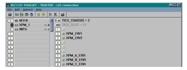
**Figure 5 Module Configuration**
